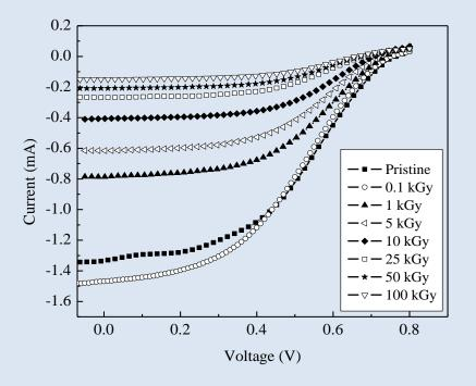
Illuminated I-V characteristics of CdTe/CdS solar cell at various doses of 8 MeV electrons
