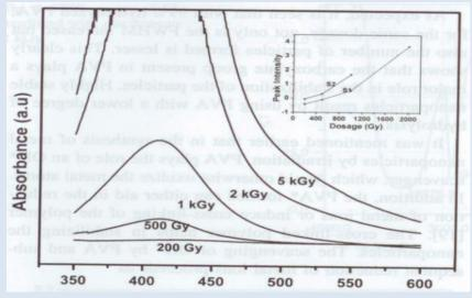
Absorption spectra of AgNO3:PVA for different electron doses. Inset shows variation of peak intensity with dose
