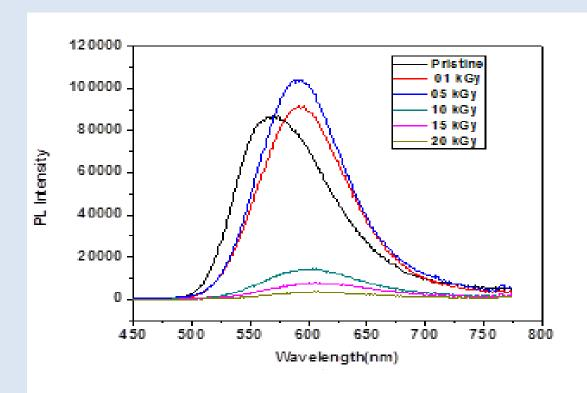
Photolumenescent Spectra of CdTe quantum dots at various electron doses
