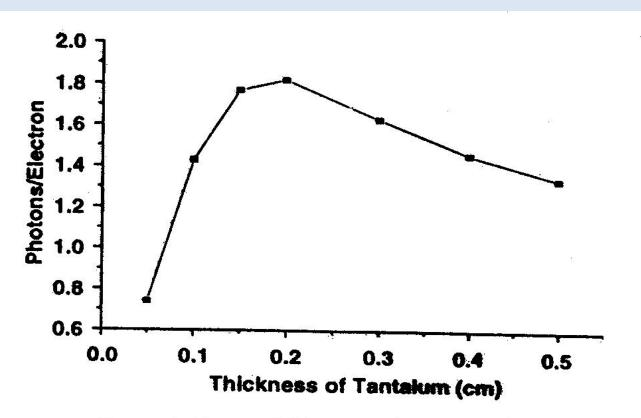
Bremsstrahlung yield for different thicknesses of tantalum for 10 MeV incident electrons.
