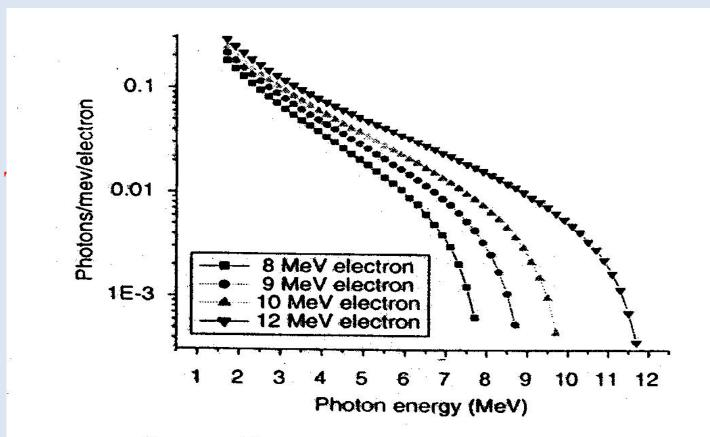
Bremsstrahlung spectrum for Ta target for electrons of different energy.
