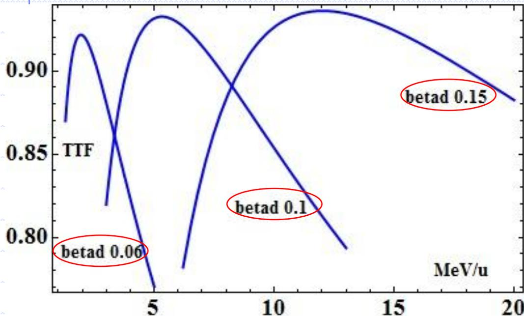
TTF of double gap QWR resonating at 100 MHz, aperture dia  $\sim 20$ mm &  $g/\beta\lambda$  ratio  $\sim 0.2$  calculated using formula described in [J. R. Delayen, NIM 212 (1983) 73-79]
