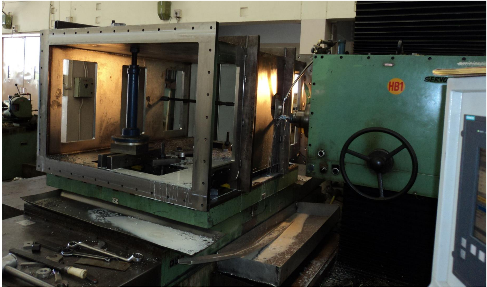
Chamber machining at CNC Horizontal Boring Machine
