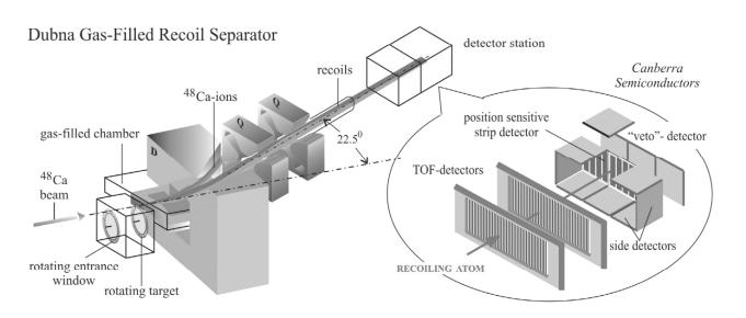
Residues are separated in a separator and implanted in the focal plane detectors
