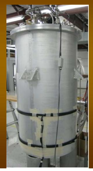
A persistent mode superconducting magnet with shim coil assembly
