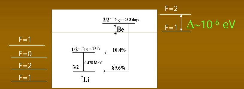
So we need to cool the system to milikelvin temperatures so thermal energy is lower than hyperfine splitting.
